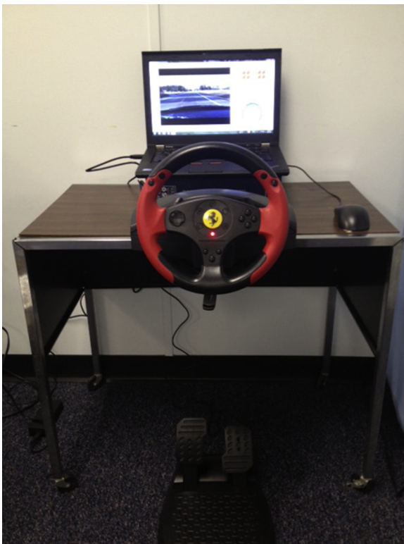
Fig. Driving simulator. The primary outcome measure of the present investigation was the mean brake response time using a computerized driving simulator. The brake response time was defined as the time from red light activation on the computer monitor, maintaining a constant accelerator speed to initiation of the brake pedal.
