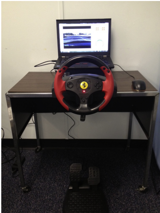
Fig. Driving simulator. The primary outcome measure of the present investigation was the mean brake response time using a computerized driving simulator. The brake response time was defined as the interval from red light activation on the computer monitor while maintaining a constant accelerator speed to initiation of the brake pedal.
